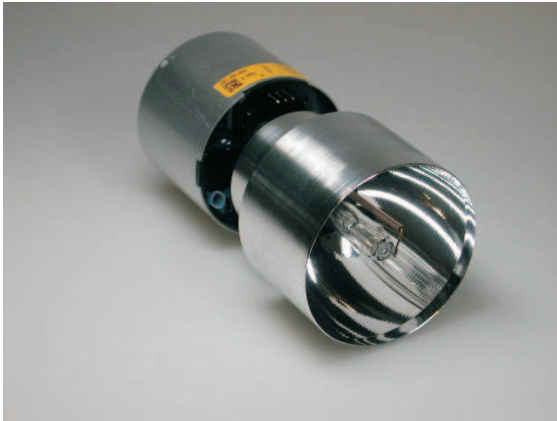
Xenon Arc Lamp Module includes balast with ignition - Ø 55x120 mm
